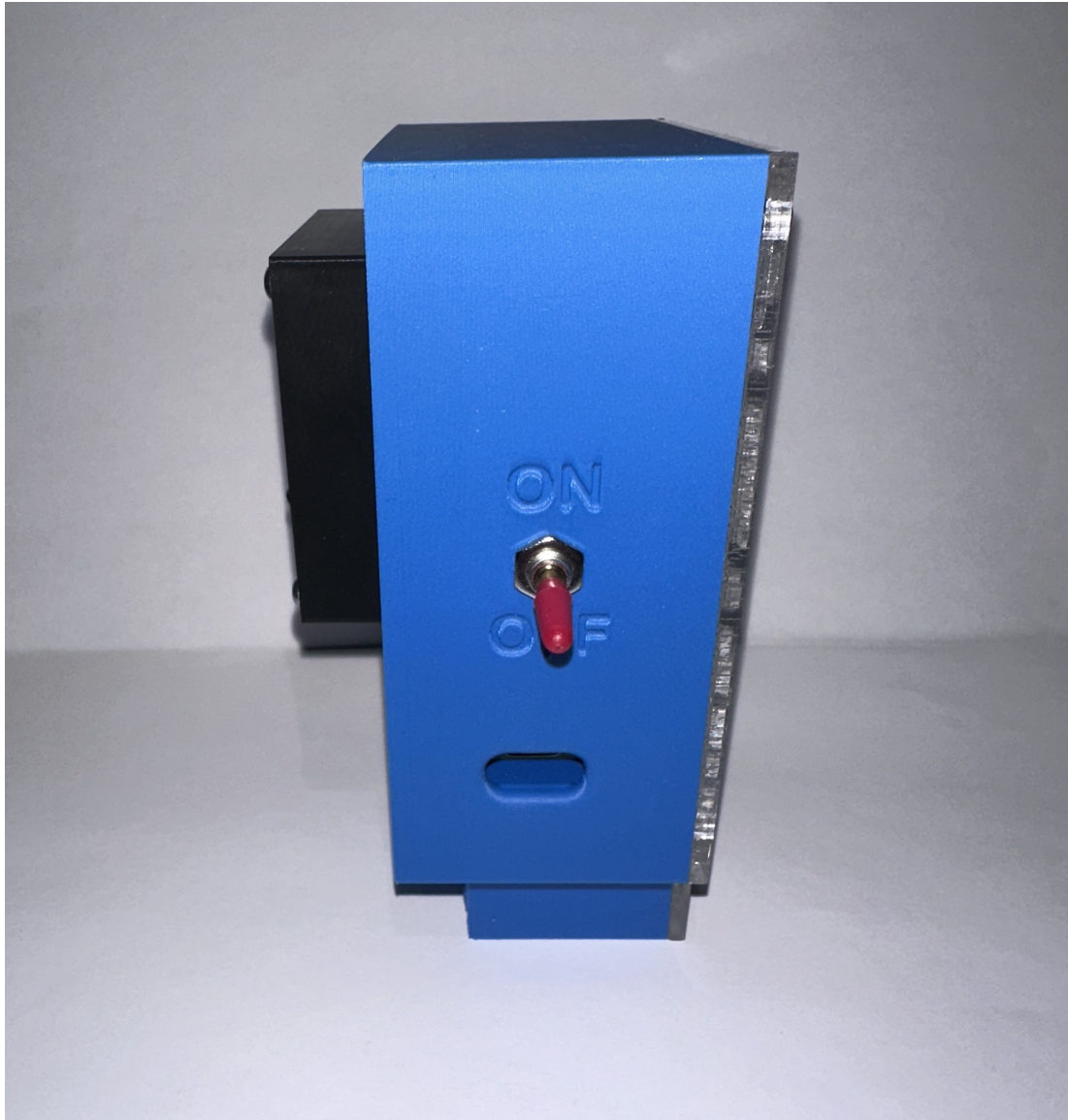
Figure B.2: Side view of the NKT_Tool prototype featuring the manual power toggle switch and charging port access.
