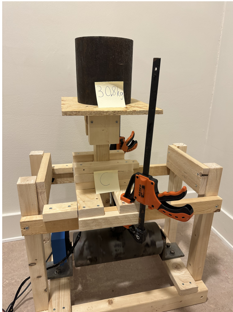
Figure A.10: Components used in the experimental setup - Roller C, 30.8 kg load.
