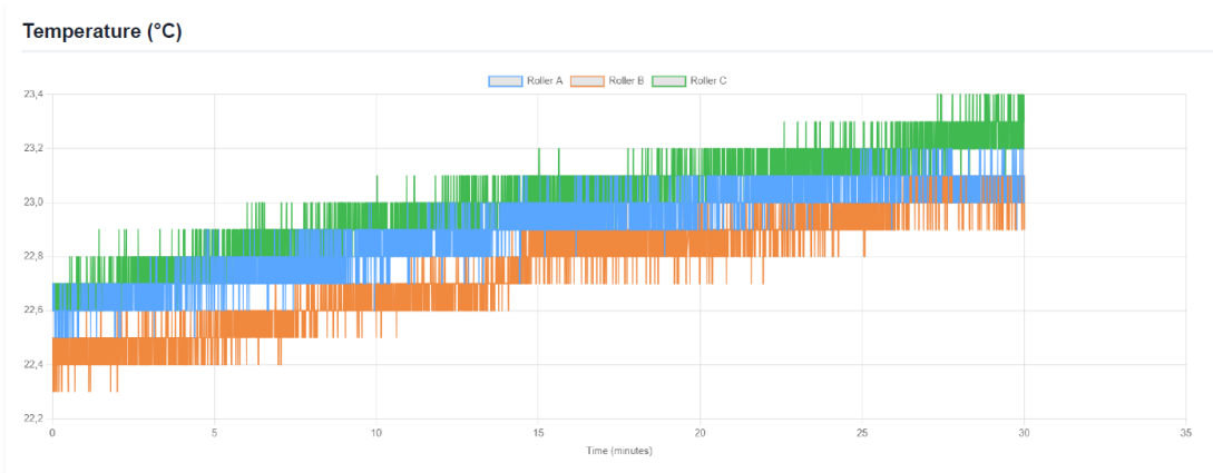
Figure C.15: Temperature trends over 30 minutes for Roller A, B, and C with a 30.8kg load.
