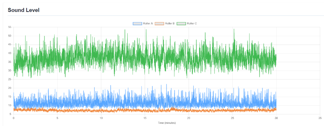
Figure C.20: Sound level measurements over a 30-minute period for Roller A, B, and C with a 44.7kg load.
