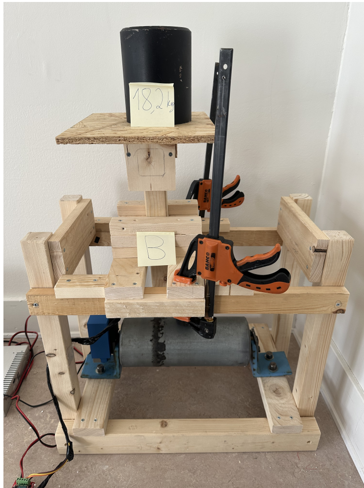
Figure A.6: Components used in the experimental setup - Roller B, 18.2kg load.
