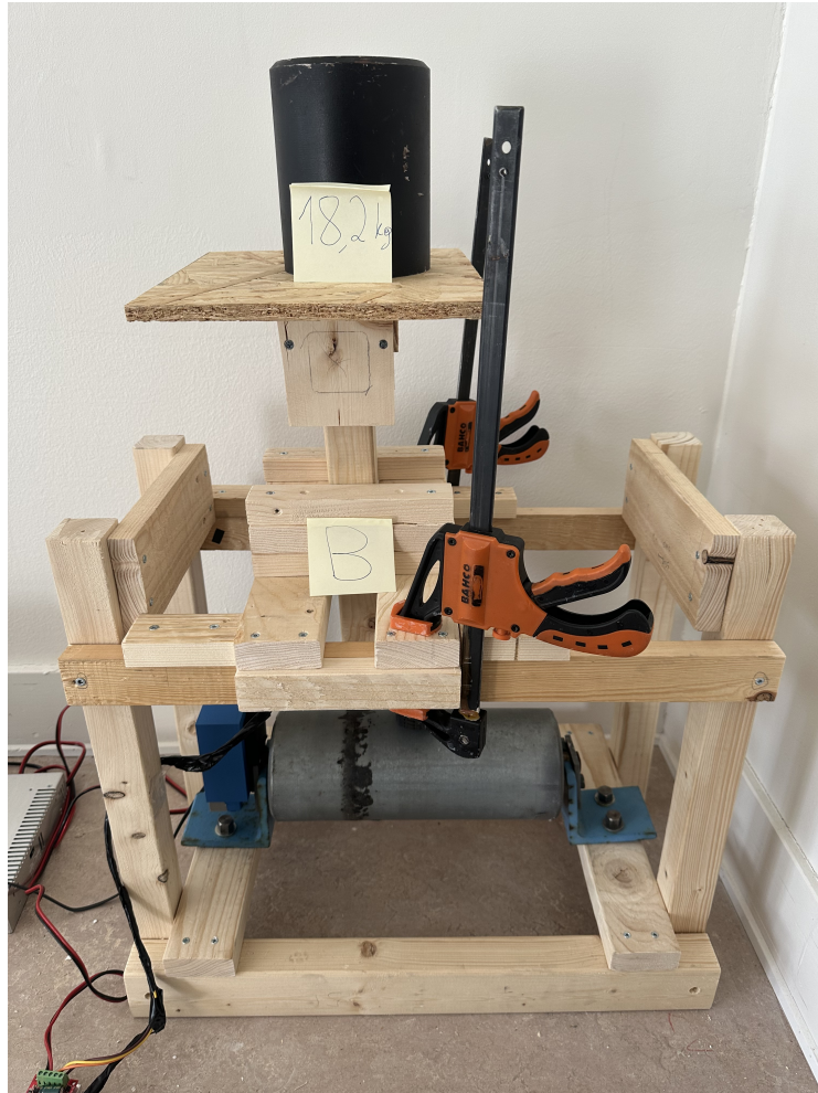
Figure A.7: Components used in the experimental setup - Roller B, 30.8kg load.
