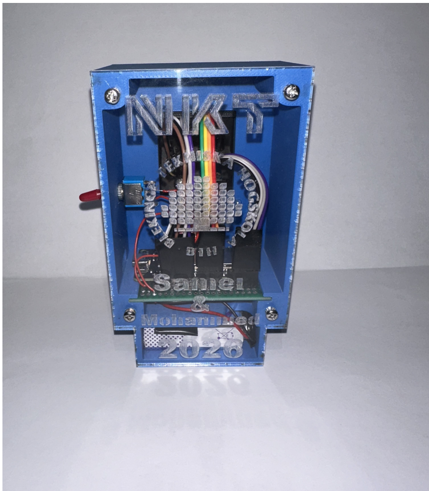
Figure B.1: Front view of the assembled NKT_Tool showing the internal electronics, LED display, and transparent casing.
