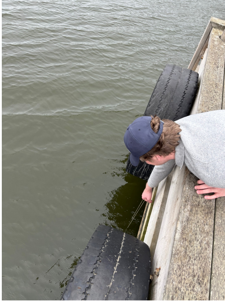
Figure 5.3: Execution of the pressure resistance test, where the AUV hull was submerged using a tethered line to evaluate sealing performance under increased external pressure.
