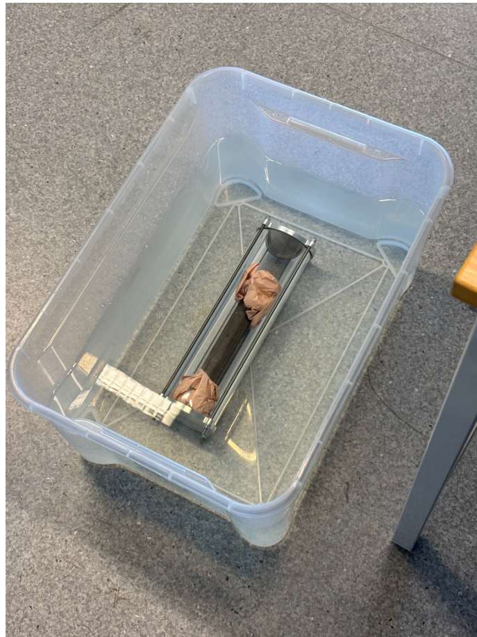
Figure 5.1: Initial watertightness test of the central hull section.
