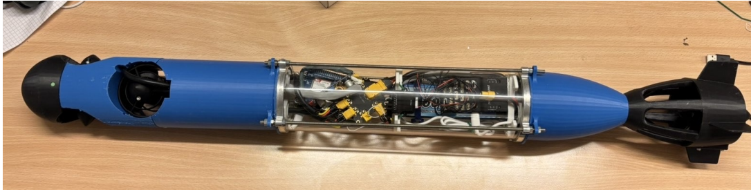
Figure 4.5: Final prototype of the developed AUV showing the modular hull structure, transparent electronics compartment, and integrated propulsion system.
