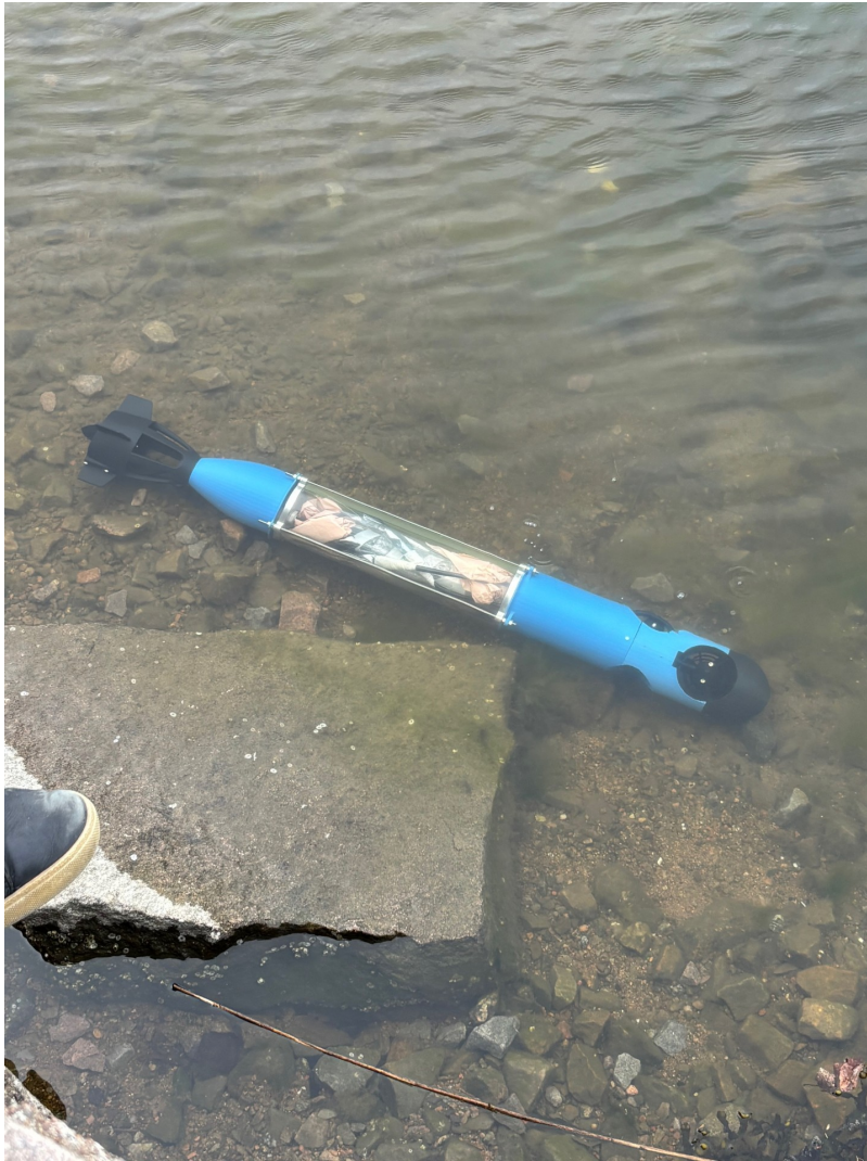
Figure 5.2: Watertightness testing of the assembled AUV hull with all cables during submersion.
