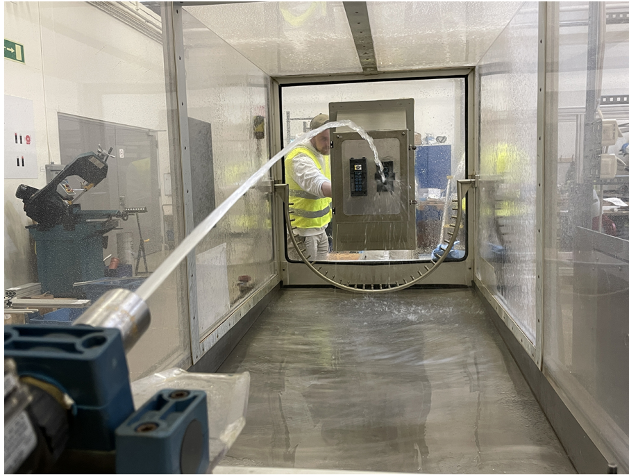
Figure 5.59: Concepts 1:2 and 5:2 in the testing environment during IP-X5 test
