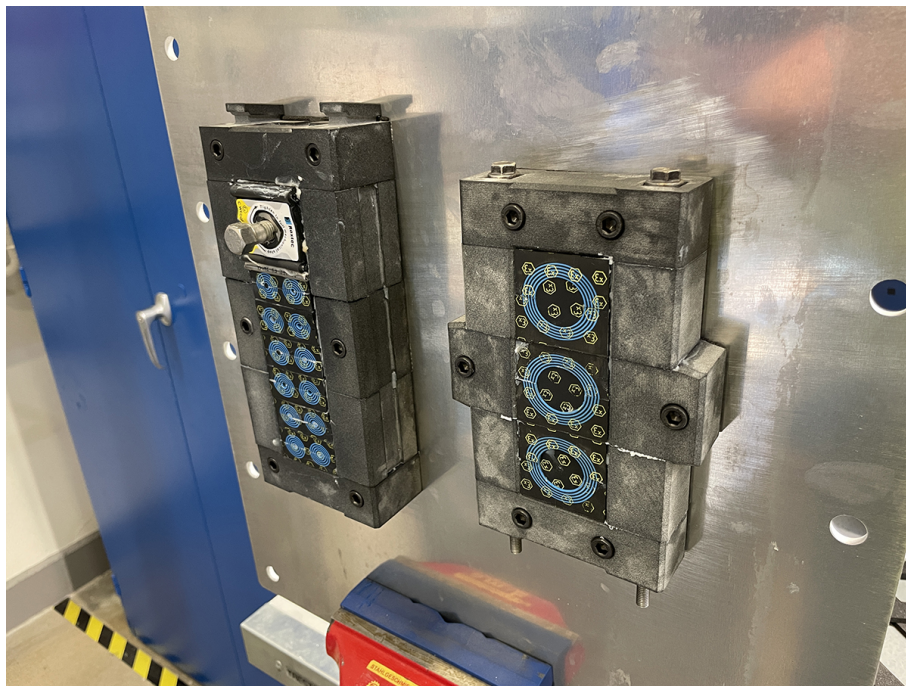
Figure 5.58: Assembled functional prototypes of concepts 1:2 and 5:2 attached to testing sheet
